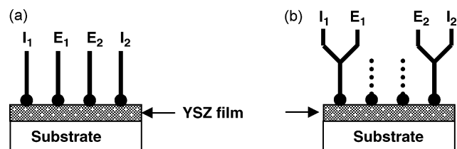
Fig. 2. Scheme of the four-electrode (a) and two-electrode (b) experimental set-up. The probes are equidistant.
